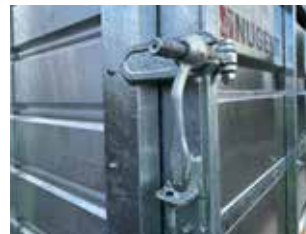
Robust taildoor fastener. Winders are simple but effective and help to strengthen the trailer when the ramp is closed.
