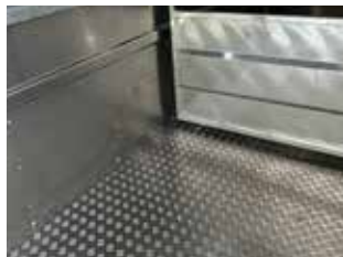
33mm timber floor with a one piece, fully sealed 2mm aluminium tread plate floor covering.
