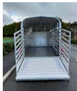
Reinforced loading ramp.
