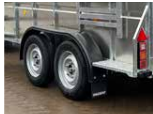
Wheels: bigger surface area tows better in fields and gives extra stability on the road. Less rolling resistance, gives a better fuel efficiency & reduces the pull on the towing vehicle.
