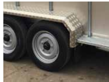
Aluminium mudguards for twin axle models.
