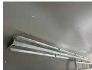
Multiple dividing gate hangers for tailored sectioning of each load.
