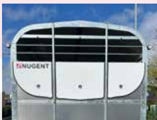
Nugent's unique trio of fold down front panels allow farmers to control the level of air flow through the trailer. This reduces drag to provide for a better towing trailer, while significantly decreasing fuel consumption.
